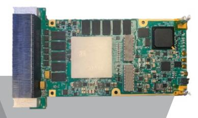
8 Simultaneous wideband TX and RX Channels with on-board processing
